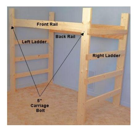
Lift the unit to its upright position. From the front insert a 5-1/2 In. carriage bolt into the hole in each of the front legs. From the inside place the front rail between the front ladder ends, the ledge must be facing inside and at the bottom of the front rail. Place a washer, lock washer and nut on each of the bolts and loosely hand tighten the nuts.
