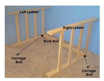
The Front Rail And Back Rails are exactly the same. From the back insert one 5-1/2 In. carriage bolt into the hole of each back leg. Lay the ladder ends on their backs as shown on right. Lay the back rail between the ladder ends. The back rail is positioned with the shorter side above the bolts and the longer side below the bolts. Place a washer, lock washer and nut on each of the bolts and loosely hand tighten the nuts..
