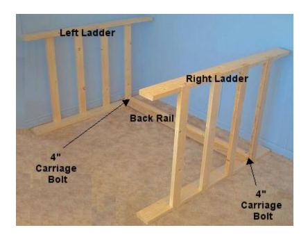
From the back insert one 4 In. carriage bolt into the hole of each back leg. Lay the ladder ends on their backs as shown on right. Lay the back rail between the ladder ends. The back rail is positioned with the shorter side above the bolts and the longer side below the bolts. Place a washer, lock washer and nut on each of the bolts and loosely hand tighten the nuts..
