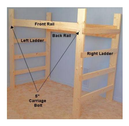
Lift the unit to its upright position. From the front insert a 5 In. carriage bolt into the hole in each of the front legs. From the inside place the front rail between the front ladder ends, the ledge must be facing inside and at the bottom of the front rail. Place a washer, lock washer and nut on each of the bolts and loosely hand tighten the nuts.
