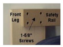
Fasten the back rail to the back legs with four 2-1/2 In. screws at each end. Fasten the front bed rail to the front legs with four 2-1/2 In. screws at each end. Note: the back and front rails are the same. Place your mattress support and mattress on the loft. Attach the 2 In. x 4 In. Safety Rail to the front and back post with the 2-1/2 Coarse Screws provide. If you ordered the youth safety rail options, you will get 2-Safety Rails for 3-Sides of the bed.
