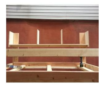
Place the Two  $(3/4" \times 7" \times 11-34")$  Center dividers in place and screw from under the Horizontal Ply installed in step above. Use the Black 1-5/8 Course Screws.
