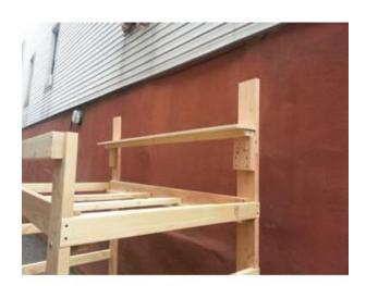
Place the bottom shelf (3/4" x 7" x 79" Ply Board) (Note: For Queen Size and Extra Long it will be 80". For Dorm XXL It will be 84") on top of the (2x4) shelf support installed in above step. Screw the Ply shelf into the (2x4) support on tight with the Black 1-5/8" Course Screws.
