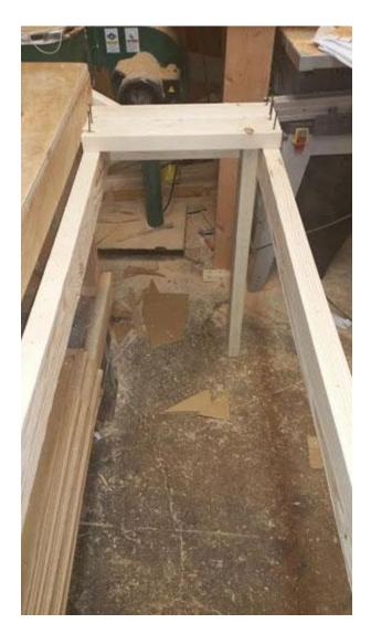
Step 3. Assemble the two (2) ladder legs and the stair stretchers.
