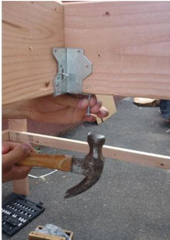
Start to connect the two separate beds, you have just made, using the Metal Angle Bracker. Hammer the 12 1-1/2 In. Galvanized Nails through the holes in the metal. Attach the horizontal stabilizer bar parallel to the bottom stair as shown in the lower part of the picture using the 2-1/2 In. Coarse Screws provided.
