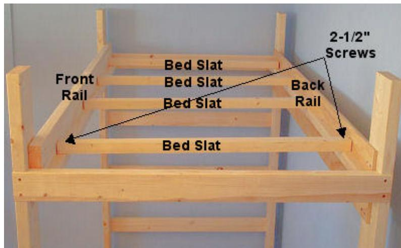
Insert the bed slats between the front and back rails, evenly spacing them apart. You can now completely tighten the carriage bolts. Fasten the bed slats to the front and back rails using 2-1/2 In. screws.
