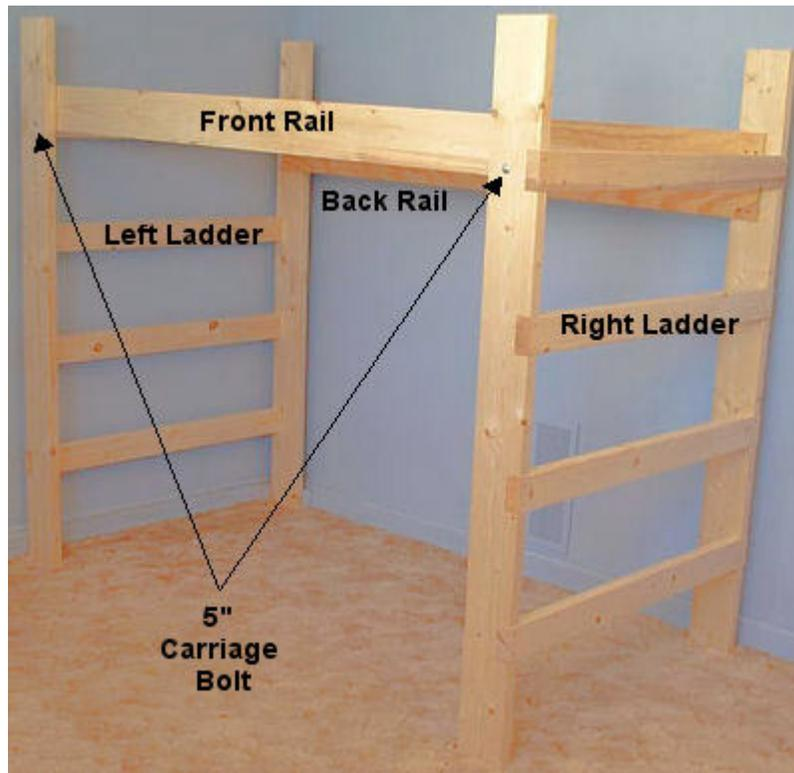
Lift the unit to its upright position. From the front insert a 5.25 In. carriage bolt into the hole in each of the front legs. From the inside place the front rail between the front ladder ends, the ledge must be facing inside and at the bottom of the front rail. Place a washer, lock washer and nut on each of the bolts and loosely hand tighten the nuts.
