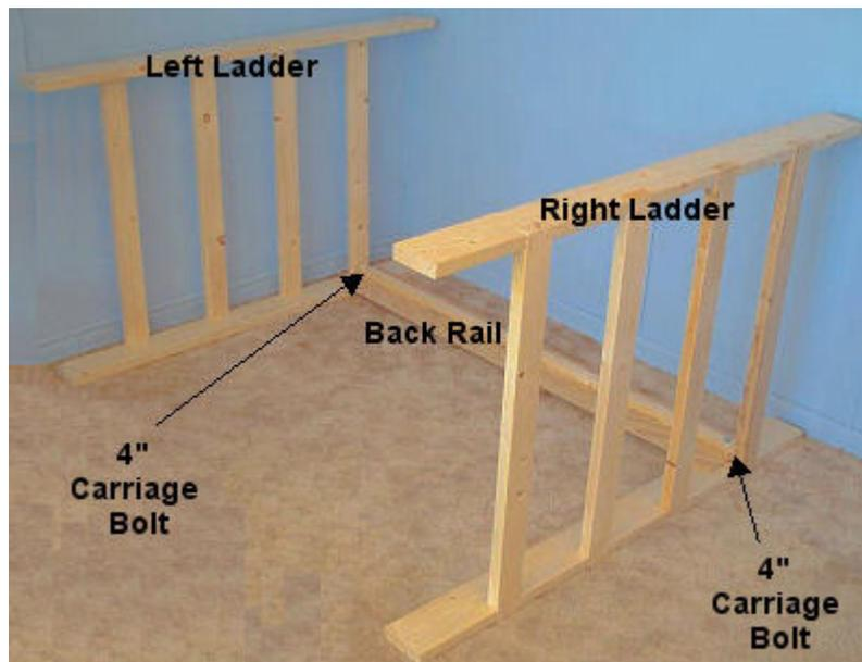
From the back insert one 5.25" carriage bolt into the hole of each back leg. Lay the ladder ends on their backs as shown on right. Lay the back rail between the ladder ends. The back rail is exactly like the front rail. Place a washer, lock washer and nut on each of the bolts and loosely hand tighten the nuts..
